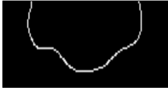
Figure 13 Edges detected after applying canny edge detection on figure 9 (b)
