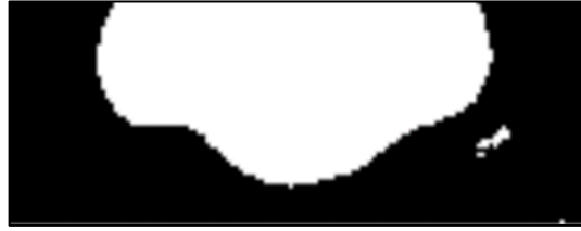
Figure 9 Segmented search area using Otsu's thresholding
