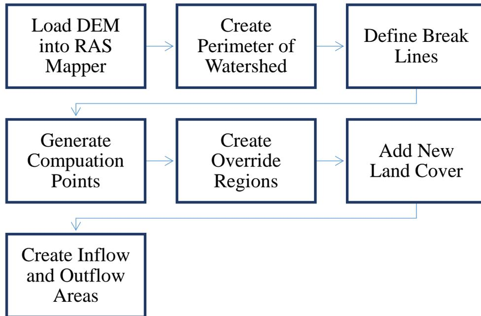
*Figure 5.2 Process of processing 2-D flow area in RAS Mapper*
