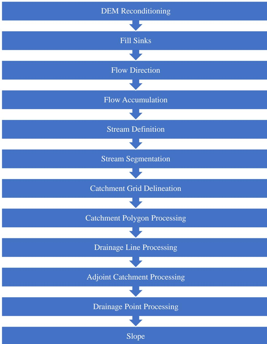
*Figure A.1 Process of running Arc Hydro*
