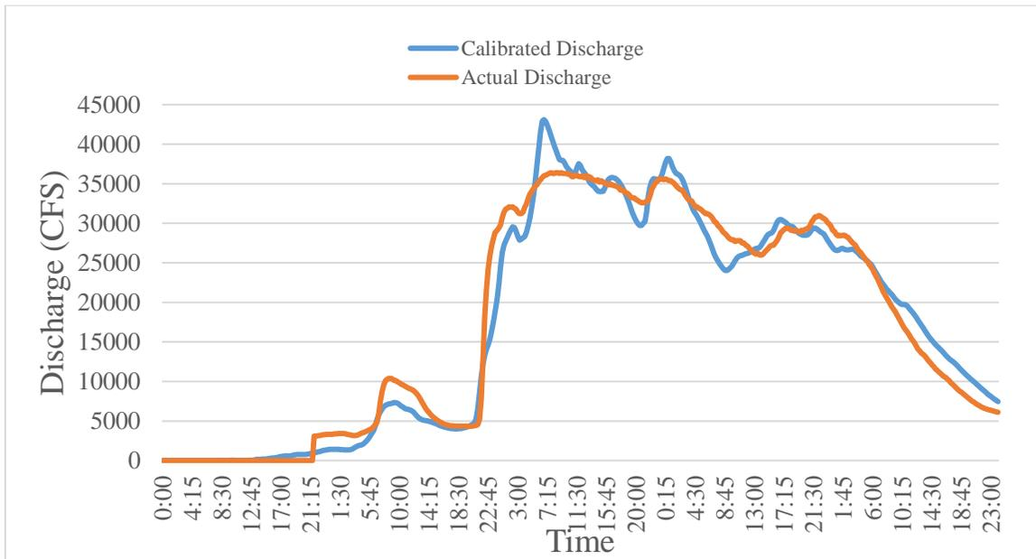
Figure 4.10 Calibration versus actual discharge of Hurricane Harvey at Junction 9
