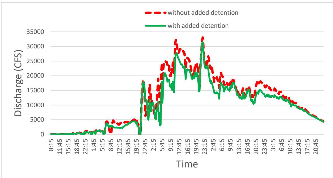
Figure 6.4 Simulation of Hurricane Harvey at Junction 115 with and without proposed detention of Westwood and Breaburn ponds
