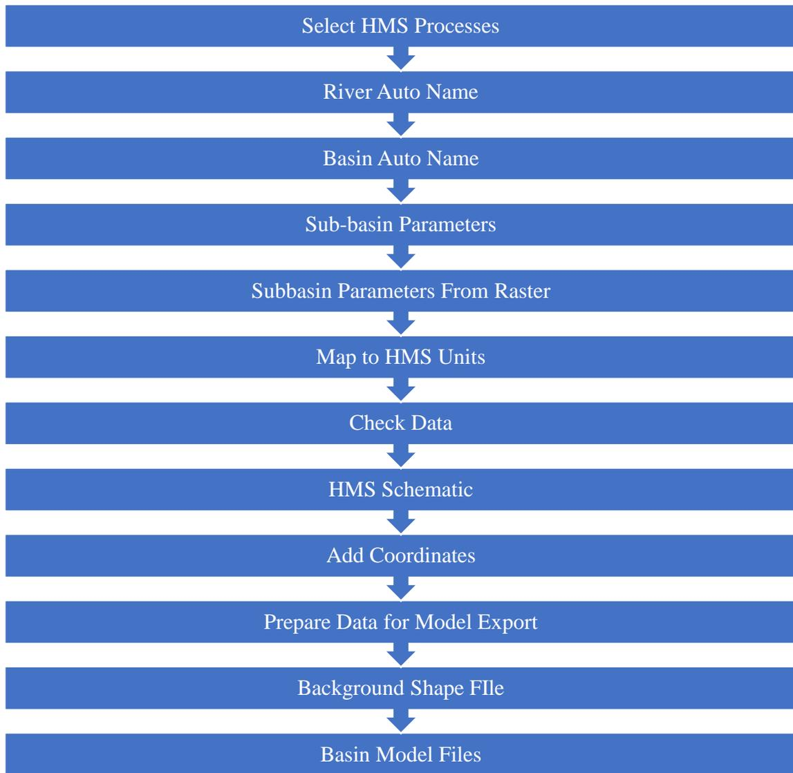
*Figure A.4 Process of Setting up HEC-HMS model in HEC-GeoHMS*
