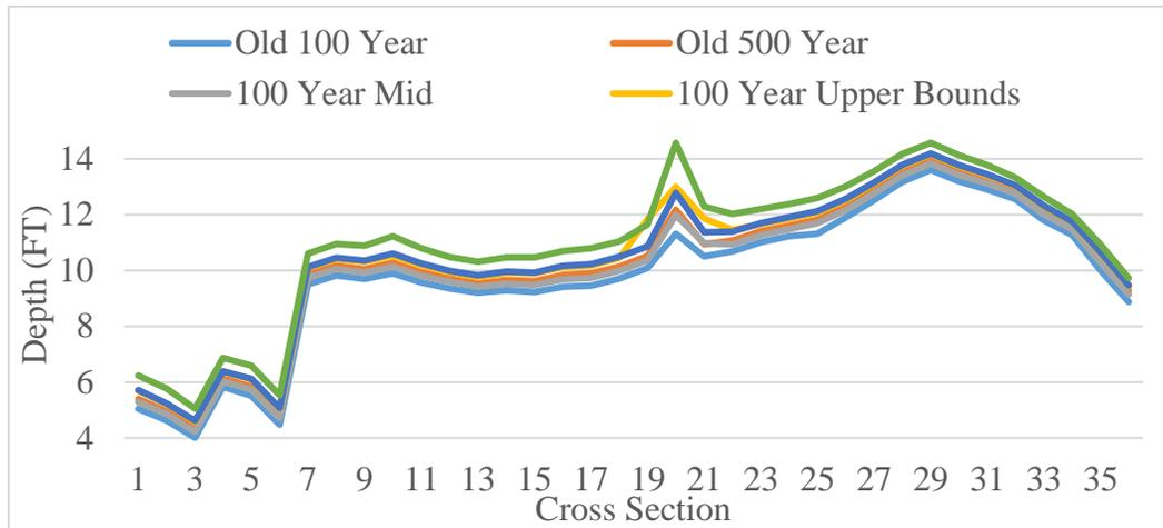
Figure 6.9 Graph Comparing the depth at the stream of all rainfall events, with cross sections going from upstream to downstream.
