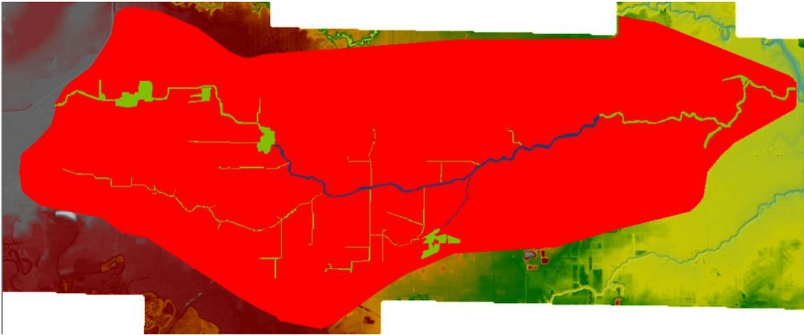
Figure C.3 Manning's N Value map of Brays Bayou Watershed. Yellow is equal to .025, blue is equal to .015, red is equal to .05.
