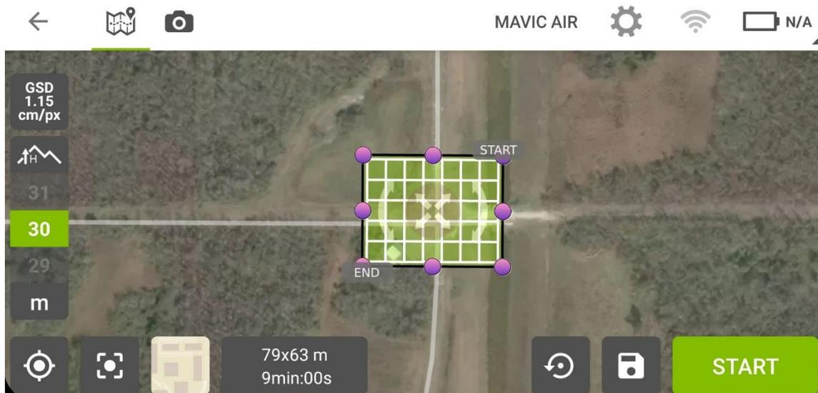
Figure 4.6 Selecting Area to be measured in using PIX4D app
