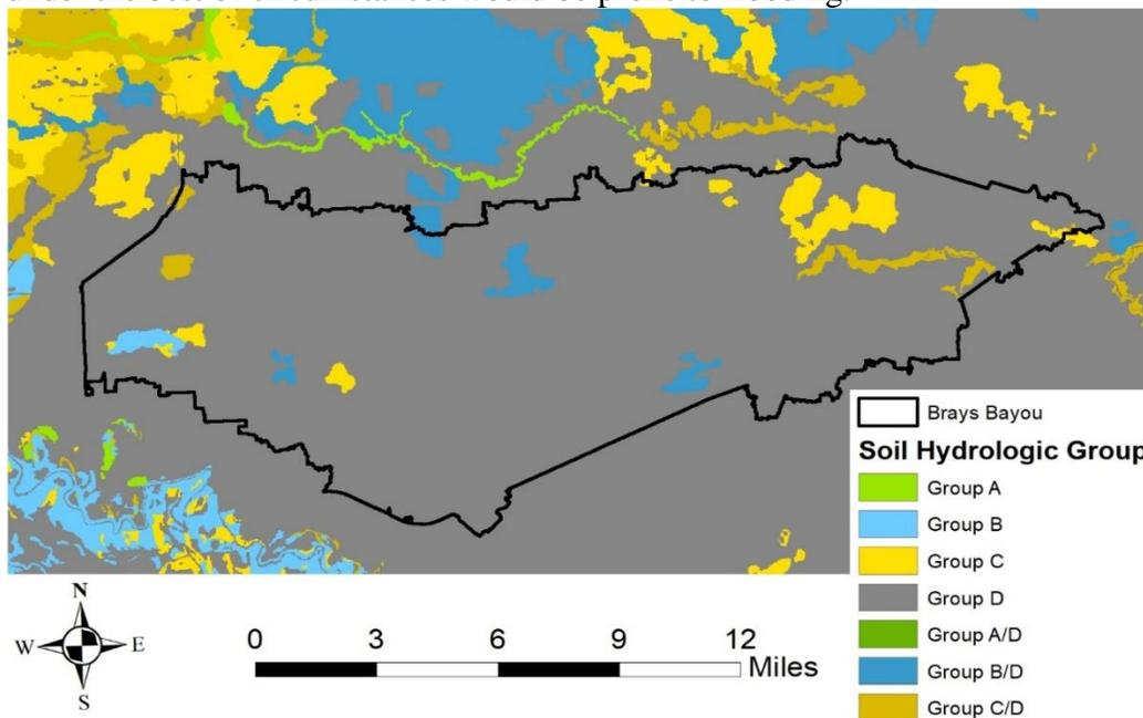
*Figure 3.3 Soil Hydrologic Groups of the Brays Bayou Watershed*
