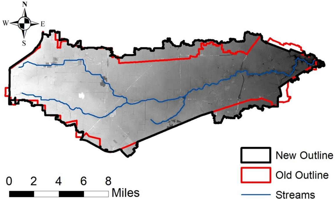
Figure 6.1 Comparison of the accepted old outline to the outline determined from the watershed delineation in Arc-Map
