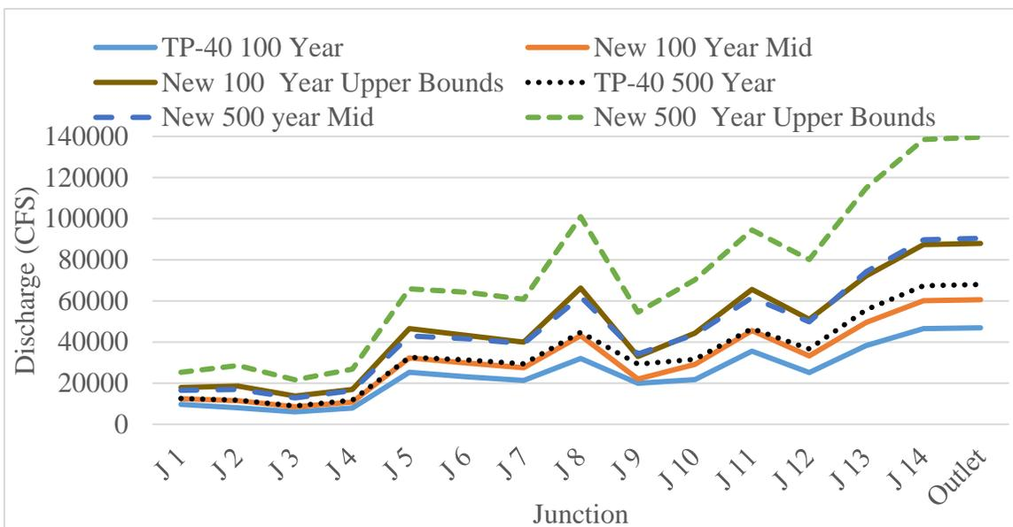
Figure 6.3 Change in Discharge at junctions within Brays Bayou from west to east.
