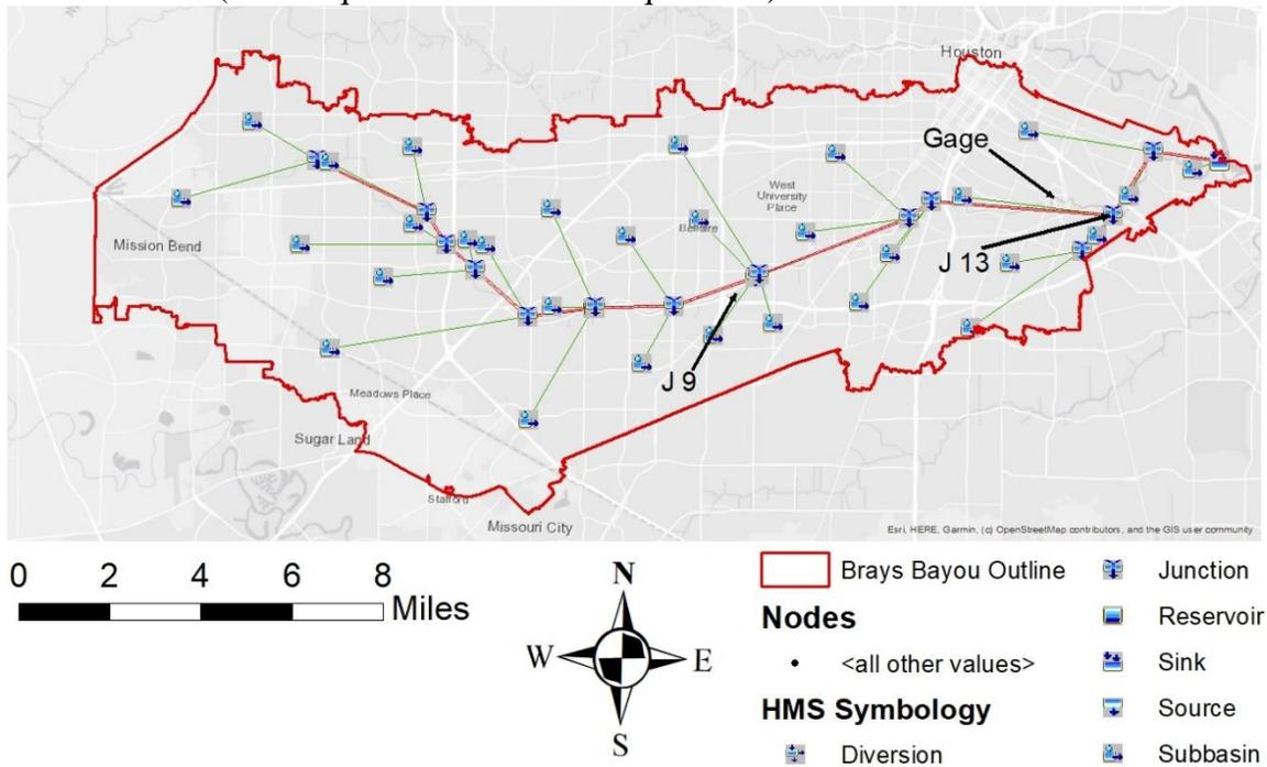
Figure 4.8 Location of J 9 which was used for determining discharge reduction for mitigation measures, and location of J13 which used for calibration.
