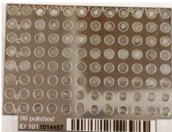
*Figure 12. Steel target used for MALDI-TOF MS. This is an example of the target used to spot samples for MALDI-TOF MS and used for mass spectrometry.*
